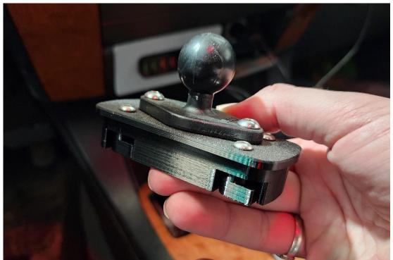
Make sure your bracket looks as shown, all the cams should be tight to the body and the Ram Mount secured ontop
