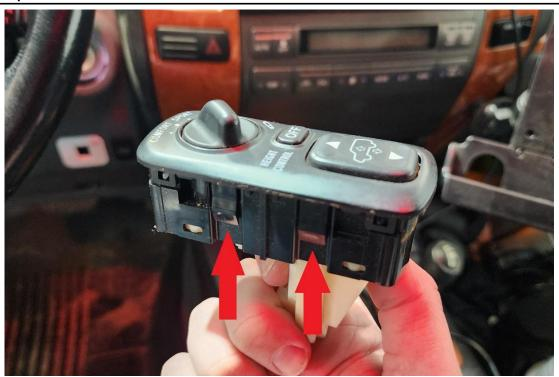
The tabs that need to be released to remove the unit, once removed undo the bottom connector plug to remove from the center console
