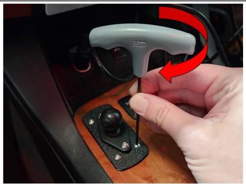
With a swift motion "flick" the bolts clockwise, this will cause the cams to spin out and lift up to secure the bracket to the panel. Once you flick it out you'll be able to tighten each one
