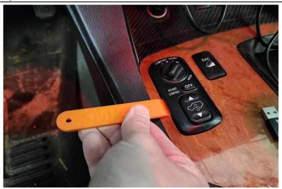
Use the Provided panel tool to remove the height control. There are 4 tabs that need to be released (see next image). You will need to pry softly between the wood and height control.
