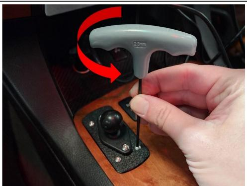
Drop the unit into the pocket and use a 2.5mm allen wrench (Tee handle prefered) to loosen each bolt. You should spin each one 3 FULL rotations to ensure they are floating freely
