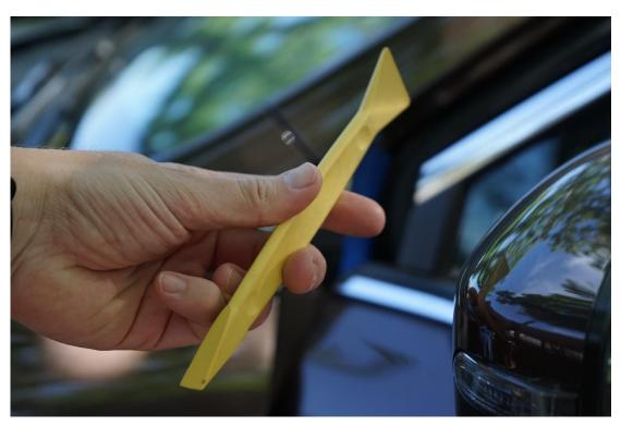
To start the install make sure you have all the mentioned tools and provided hardware. Open the door to about 60% open, put down painters tape on the painted surface next to the cover as shown. You will need to pry carefully but forcefully to pop the 3 plastic tabs free. Take your time, these can be stubborn.
