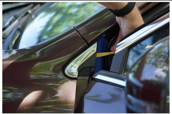
Once you are able to get the edge shown lifted you can start to "peel" the panel off the vehicle. You will feel 3 distinct pops as each of the fasteners releases\* (Outback Shown) \*There is a chance you may break one or more of the tabs, don't worry this will not effect install and can be replaced if you ever wish to go back to stock.
