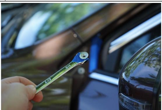
Use tape on an open ended wrench to secure the nut in order to feed under the Ditch Light Bracket. Mount the panel to the side of the vehicle and feed the bolt through the previously mounted bracket and secure with the above M6 nut. Keep this loose
