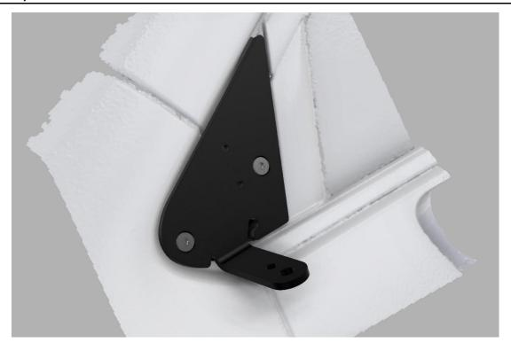
Now feed another M6 nut further in to meet the forward M6 bolt, once you have both threaded you can secure both until tight. Check the perimeter of the bracket for interference with the body. Once finshed you may add your pods and start wiring!
