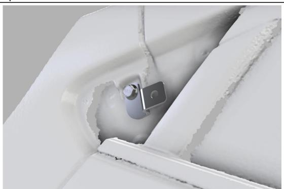
There is an M6 bolt that holes the fender panel to the body here, remove this with your 10mm socket, install the bracket as shown then reinstall the bolt and securely tighten. Final install should look as shown
