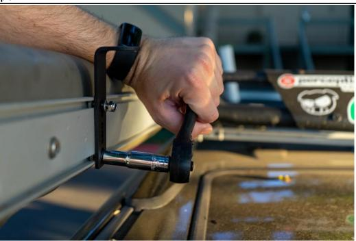
Tighten down, be sure to go just before snug, get off the vehicle and check the mount is square, once straightened out secure down. Do not over tighten!
