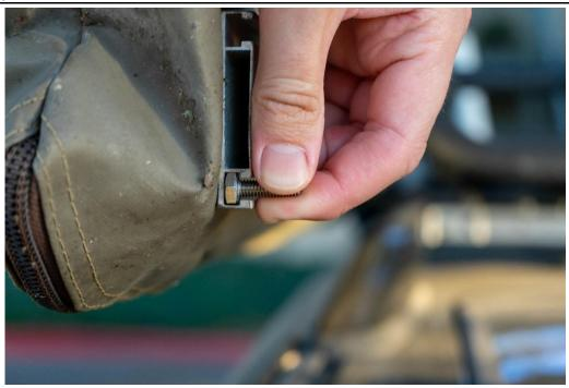
Slide the hardware into the existing mount slots, you may need to temporarily remove one of the existing vehicle mounts to slide the hardware to where you desire.
