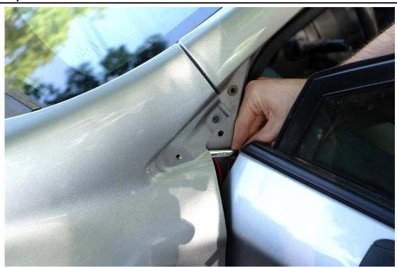
You'll find the best approach at this angle up into the fender with the door partially open, line up the nut to the forward hole (Blue) and then bring the bracket with the hardware installed up to the vehicle, thread the forward bolt by hand until it engages
