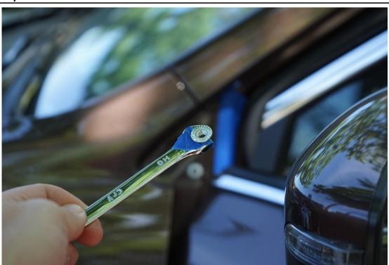
When installing the foremost bolt we will be threading into the provided nut, to best secure the nut during installation use tape to make a temporary hold on the nut, this helps ensure you don't drop it down into the fender (extra nut provided)
