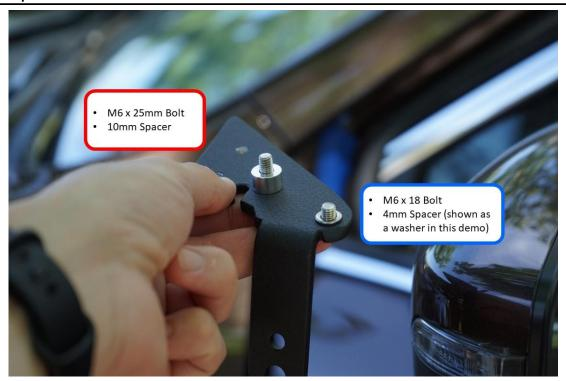
Hardware installed into the bracket as shown
