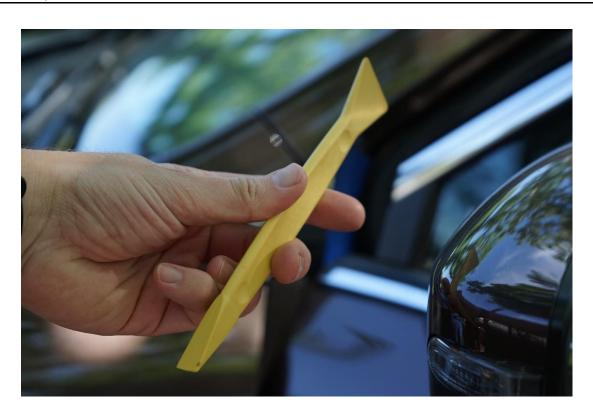
To start the install make sure you have all the mentioned tools and provided hardware. Open the door to about 60% open, put down painters tape on the painted surface next to the cover as shown. You will need to pry carefully but forcefully to pop the 3 plastic tabs free. Take your time, these can be stubborn.
