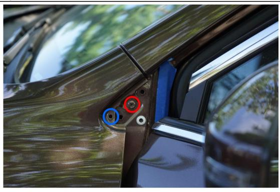
Once removed you will see an M6 bolt (red circle) that needs removed using a 10mm socket. Noted are the Red and Blue holes that we will use for the installation
