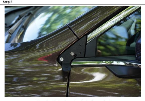
Tighten both bolts down, installation is complete!
