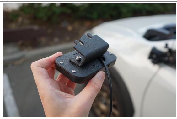
Once the angle is set lock down both M5 bolts nice and secure, then add the 4 M3 bolts to secure the panel to the plate
