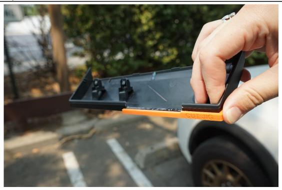
Use a dremel, razor blade, coping saw, etc to cut out the slot from line to line. See the next step for how to measure depth
