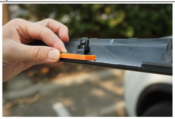
The Jig also functions as a measuring stick! Simply make sure it sits even with both side of the slot to the existing level. There is a small amount of buffer in this depth so you have room for off cuts
