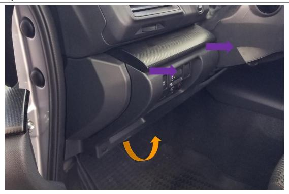
Grab the bottom (ORANGE) of this panel and pull, once the bottom is disconnected pull the panel out towards you via the PURPLE, disconnect the wires. You may need to separate the far right side
