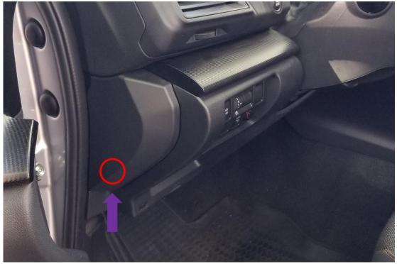
Start by using a flat head screw driver to pry the side panel off, this is held on by clips only so once it lifts pull it off by hand. Once removed there is a Philips head screw (circle in red) that will need to be removed.
