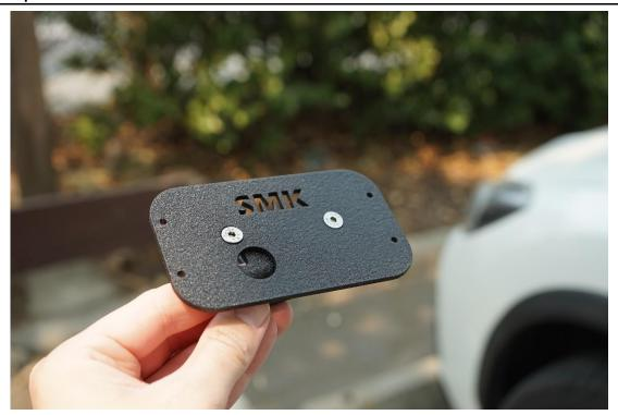
Assemble the two panels together, leave the left bolt loose/snug as this side allows you to index the angle you want the panel to sit. Do a mock up install by putting the dash panel partially back and inserting this assembly into the slot to feel out the angle you want. Once you find the angle you want lock down both bolts to secure the two pieces. NOTE - You will need to wire the Switch panels plug through the large hole BEFORE bolting the two brackets together.
