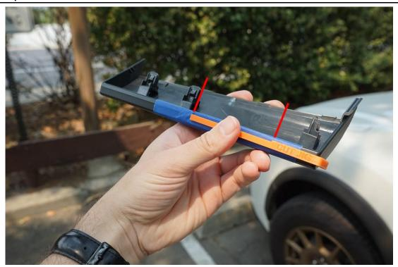
Tape the leading edge of the trim panel and place the provided Cut Jig as such, You will mark with a pen the end of the jig and the first step as shown with RED lines
