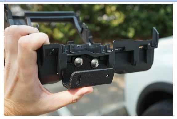
TIP - The way this will work is once the trim is back on the bent bracket get slide in between the trim and body panel. Once each carriage bolt is in one of the square slots on the bent bracket you will be able to tighten and secure the bracket in place. All this hardware will be hidden!
