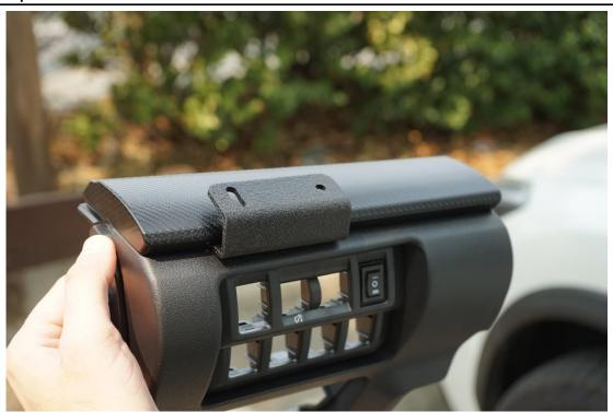
To get the bracket in the slot you'll want to slowly guide it in until it either catches on the carriage bolts or slide into the slot. To make this fit you'll want to grab the carriage bolts from the inside of the dash and slightly twist/jiggle to help align both. When the bracket is all the way in it should look like the above image. Don't tighten this down just yet, we need to get the Switch Panel installed
