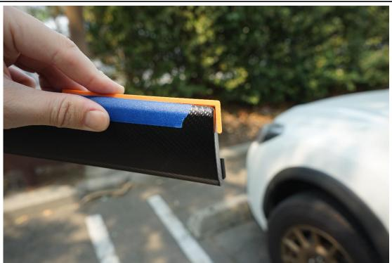
When setting up the JIG make sure the short leg is up against the side of the trim. Please double check you are cutting the correct side of the trim piece, its easy to get confused when the trim is upside down, mirror my images for accuracy
