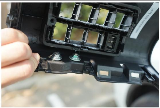
Place a washer and nut on each carriage bolt, be sure to leave these loose for the next steps
