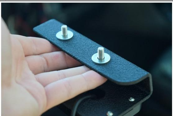
Install the carriage bolts from inside the bracket, plate the smaller of the 4 washers ontop of the bracket as shown.
