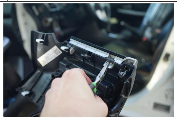
With the panel off locate the two tabs for the factory trim, using plyers bend the tab down so you can slide the tabs through the dash
