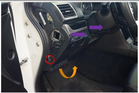
Once open remove the bolt in RED, then grab the bottom (ORANGE) of this panel and pull, once the bottom is disconnected pull the panel out towards you via the PURPLE, disconnect the wires
