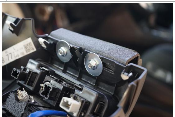
I find it best to hold the bracket like in the last image and lower the dash piece onto it so the bolts and washers stay in place. Once the bolts are through the holes add the oversized washers and lock nuts. Tighten slightly, you can move the bracket a tad then tighten down once straight
