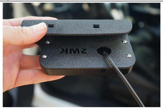
Secure the switch panel to the bracket via the 4 provided button screws. You may need to use a ball allen wrench for the back 2 bolts. Don't need to go overly tight, just snug
