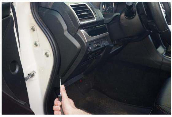
Start by using a flat head screw driver to pry the side panel off, this is held on by clips only so once it lifts pull it off by hand
