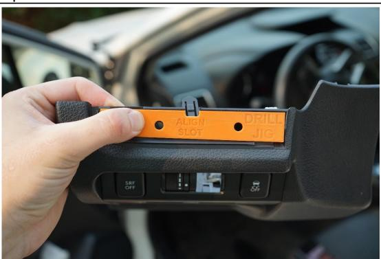
Use painters tape or something to mark the plastic to drill, lay the provided template over the area. You'll want to align the center slot with the one on the panel, push slightly up and to the right so it sits against the lip. This will be the location to drill the holes.
