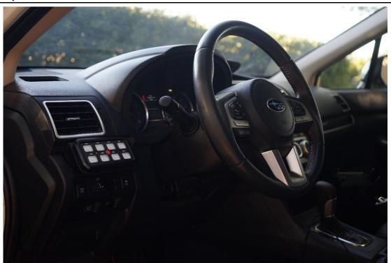
Reinstall the dash piece, check the bracket is how you want it, if you find you need to adjust it you can try to loosen the nuts and adjust, if you still need more then use the drill to slighly open the holes to allow a little more wiggle room. Route the wire through the dash and you are good to go!
