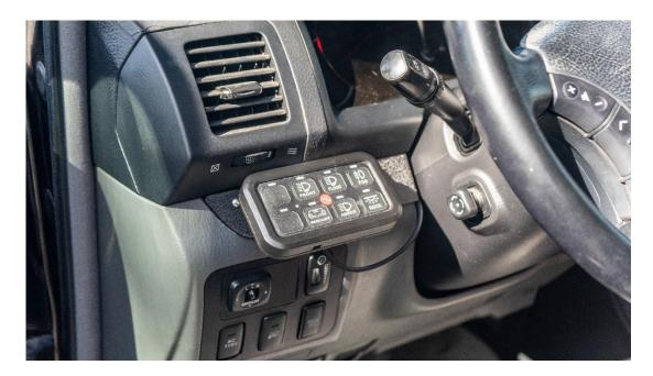
Now insert the long M6 bolt through the hole on the right side of the panel and thread till tight. It won't sit flat on the surface but this will not cause any issues! You can slightly adjust the position it sits so use this time to tuck the panel up against the upper trim
