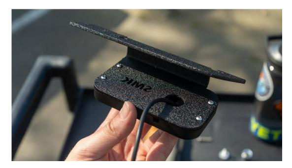
Now bolt the switch panel to the bracket with the provided M3 screws. Use the provided 2mm allen key as the rear 2 are in a tight spot. Alignment of the panel to the bracket will only go one way
