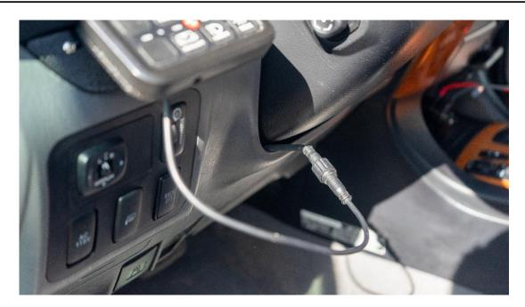
Once install connect to the wire that was fed through the firewall, twist the lock tight and tuck under the steering wheel (see Step 6 image for final wire fitment)
