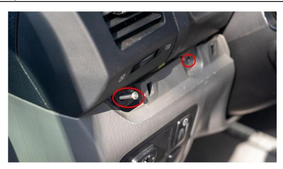
Hand thread the M4 bolt (smaller of the two provided) into what was the vent bolt (the thread are different, this bolt is only being used to stop rotation, not a securing fastener). You want to leave it mostly exposed at this point
