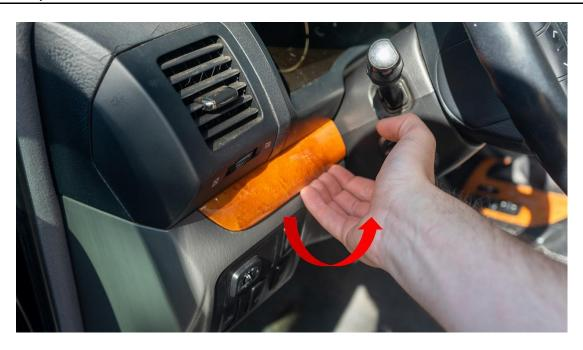
To remove the trim either use your hand or a soft plastic pry tool to lift the panel off the dash
