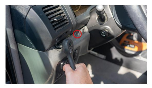
Remove the vent bolt (10mm Socket) as well as the M6 bolt holding the dash to the gauge cluster (circled RED)
