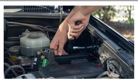
Begin fastening both bolts, be sure to not completely tighten one before both are barely snug. There is a slight amount of adjustment to get the bracket level to the engine bay
