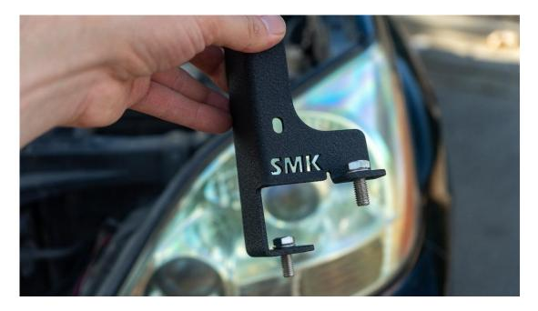
Place one M8 bolt and washer as shown into each of the side mount holes
