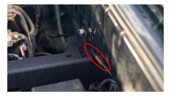
There is a cable that passes through this mounting location, be sure to not pinch it, it will sit freely through the bracket as shown once the bracket is tight
