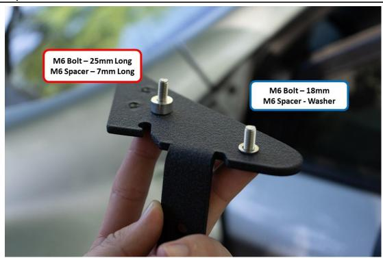
Above is how the hardware should be installed on the bracket
