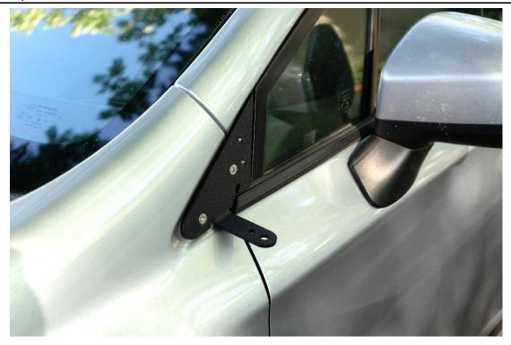
Once you have tightened the forward bolt remove the wrench from behind the fender and begin to tighten the rear bolt that goes into the frame. When both bolts are tight you can begin to reassemble
