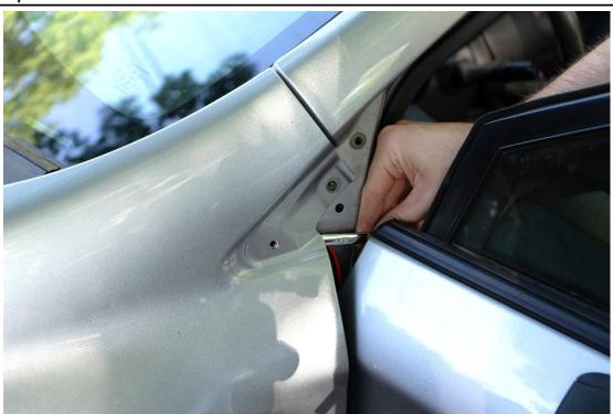
With the nut behind the fender and lined up with the forward hole begin to thread the ditch light bracket into both holes. Once you have the thread engaged on both simply begin to tighten the forward bolt first
