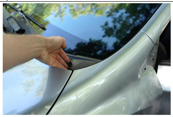
At the end of the windshield cowl are covers, these are only held in via clips, lift up as shown to pop out the panel on the side you are working on
