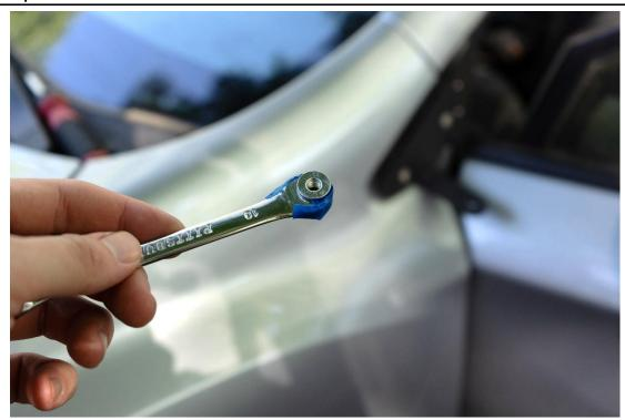
This operation is tricky so I advise using tape or other means to secure the nut to the wrench. This will help hold it in place until you get it threaded onto the bolt. I have inlcuded an extra nut just in case but if you need more you are looking for a Stainless M6 lock nut
