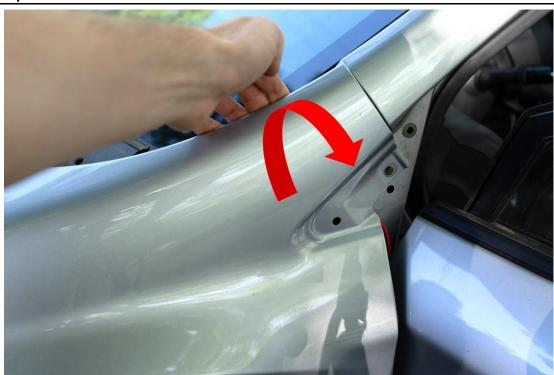
With both fender bolts removed it is time to install the bracket. Grab the top of the fender as shown and slowly pull the fender forward. You are only doing this enough to open the gap under where the ditch light bracket goes to fit the wrench
