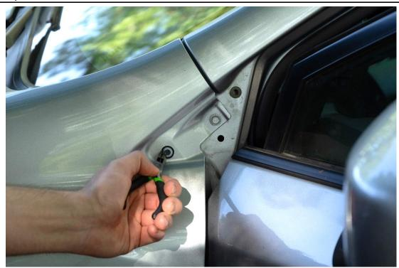
The forward fastener retaining clip needs removed, it is best to use pliers preferable needle nose. The part will be damaged while removing, it will not be salvagable.
