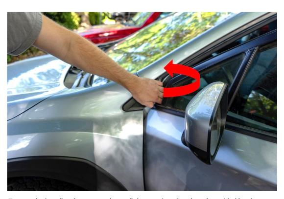
To start the install make sure you have all the mentioned tools and provided hardware. Open the door to about 60% open, grab the plastic panel as shown above and pull in a forward prying motion. This panel is secured with 3 pop fasteners so you should feel all 3 come loose
