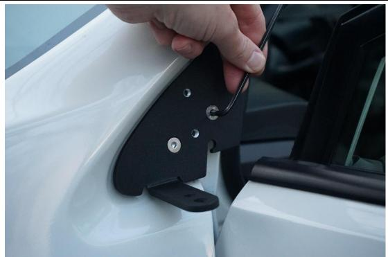
Once both bolts are threaded you can snug up both, you have a slight amount of wiggle room so make sure the bracket isn't contacting the body anywhere. Once set tighten both bolts (Do not over tighten)
