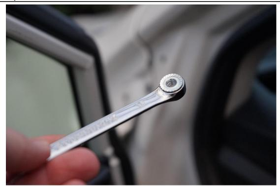
Now place the provided M6 lock nut into the 10mm wrench. It is advised to use tape or something to keep this from falling out as it is likely to fall into the fender (a spare is provided).
