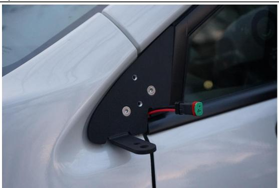
Once installed you can now run your harness through the fender (remove the felt liner in the engine bay to see through the fender).
