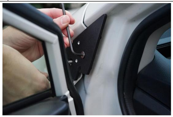
SLOWLY bring the bracket to the vehicle, be sure to keep the bracket tilted backwards to prevent the spacers from sliding off. Get the shorter bolt into the open hole. Then use the allen to engage the longer bolt into the threaded hole in the frame. Do Not tighten, leave this loose.
