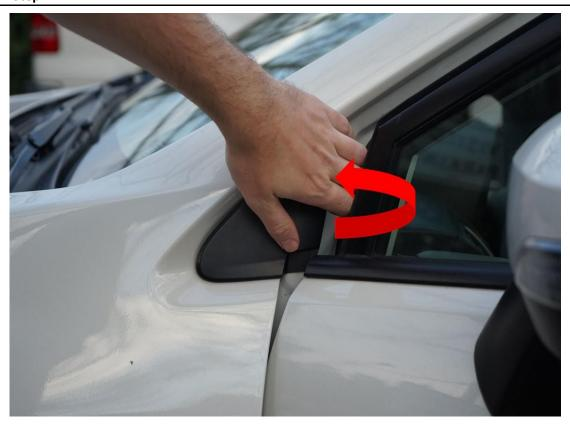
To start the install make sure you have all the mentioned tools and provided hardware. Open the door to about 60% open, grab the plastic panel as shown above and pull in a forward prying motion. This panel is secured with 3 pop fasteners so you should feel all 3 come loose
