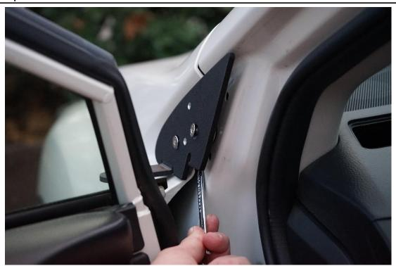
You will need to snake the wrench head up into the fender. If you can grab the shorter screw head pull it out slighly to give yourself room to get the M6 nut behind the threads. Use the 5mm allen to engage
