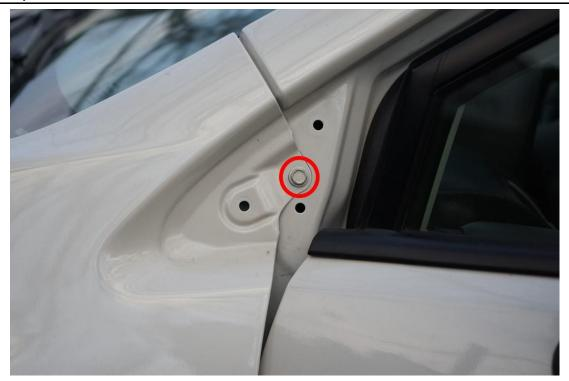
Under the panel you will find a M6 bolt, remove this with a 10mm socket and ratchet
