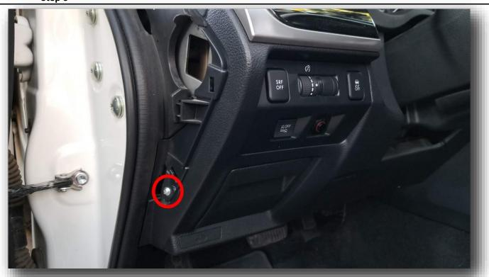
Once the panel is removed there is one phillips screw that needs removed
