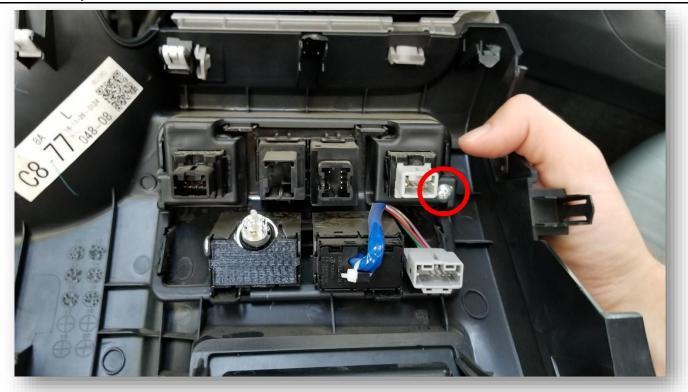
If you wish to remove the panel undo the one screw and unclip the opposite side
