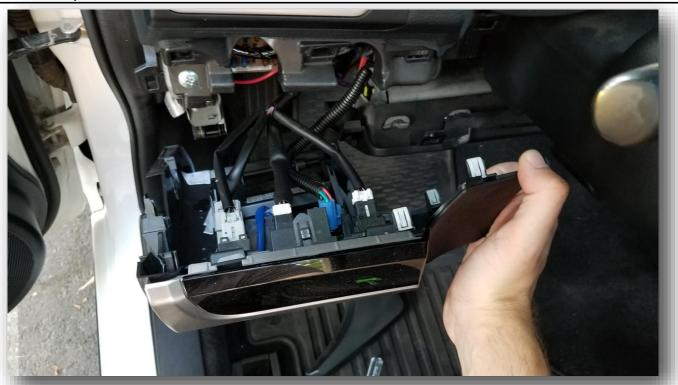
Once the bottom is loose the rest of the panel can be popped off by pulling straight out. DON'T pull too hard as any switches on the panel are still connected, they are all different so there wont be confusion
