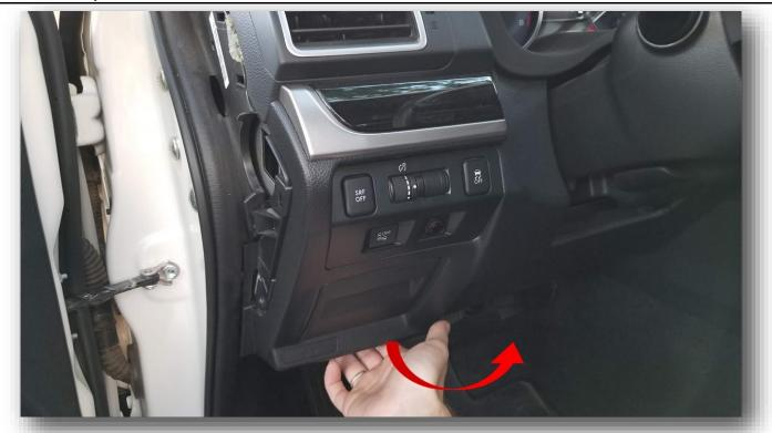
With all that removed pull the panel from the underside, do so in a swinging motion. NOTE- The Hood release is here, don't pull it by accident
