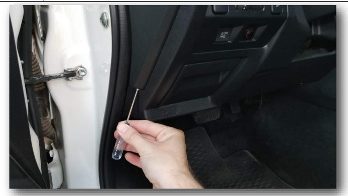
On the side of the dash you need to pry this panel off. Do so with a small or flathead screwdriver
