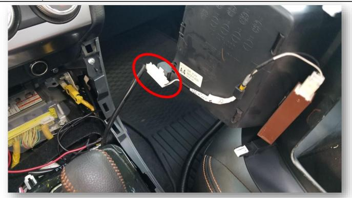
There is a plug on the back of the panel (might not be on all models) Be sure to disconnect this for an easy install
