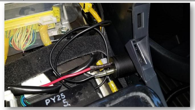
Finally connect both the pins and turn the vehicle onto aux to verify functionality. Reverse these directions to install all panels again! Congrats on an easy install!
