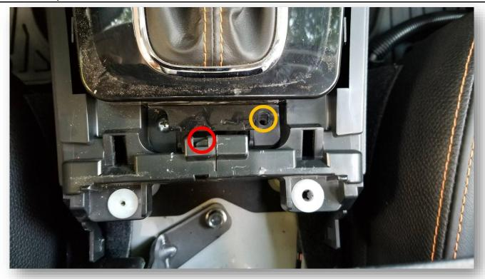
With the 2 screws from the last step removed you need to use the small screwdrive to depress this clip (in red) to unclip the two side panels from each other
