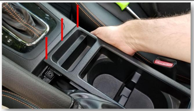
Once removed grab the plastic console by the side and lift up, it will pop up. HINT- If you need to lift this further up later in the install remove the back of the console behind the arm rest
