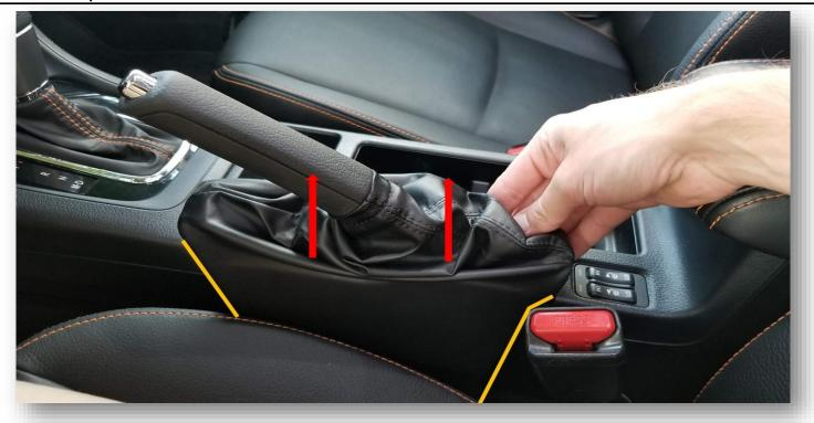
Start by removing the e-brake boot, do this by pulling strait up on the boot, you will feel it pop out of its hold
