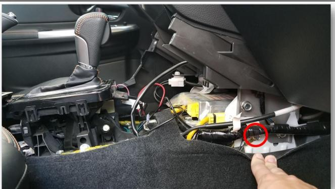
While the panel is still off undo this bolt and attached the NEGATIVE ring here, this is a common ground location so no prep is required, torque till tight again
