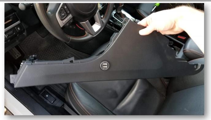
Using the template provided (or linked) install the USB outlet. This requires a 1.125" hole saw to perform
