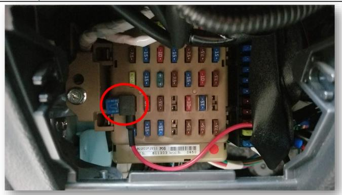
Finally connect the provided Add-a-Fuse to spot #20. This location will only provide power when the vehicle is on. If you wish to run it full time you will need to identify a constantly on fuse
