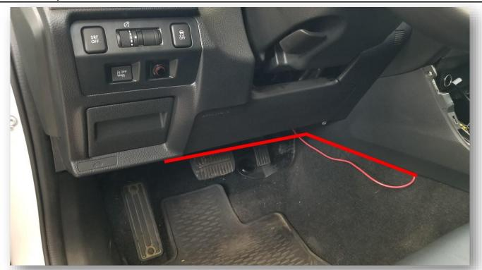
Run the provided POSITIVE wire along this route, use zip ties to secure the wire to other harnesses and tuck the side under the console side panel
